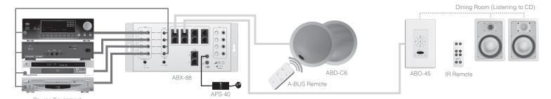
The ABX-88 Multi-Source Hub is compatible with any A-BUS room unit, either an IR Volume Control Module or A-BUS/DIRECT speaker. It is possible to mix Multi-Source Hubs with single source Hubs.
