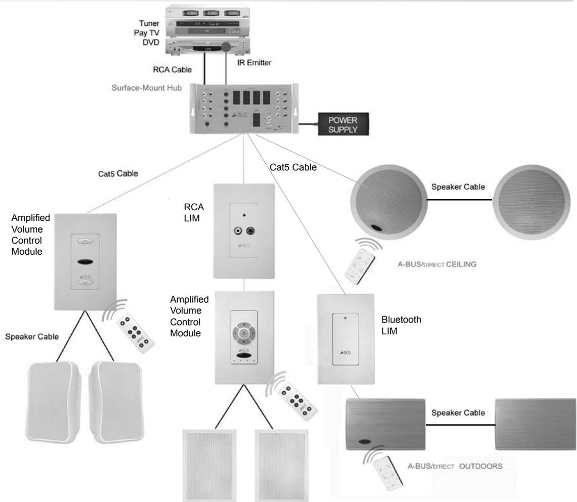
emitter connected to the IR sensor on the source component. When the system is in mute mode the infrared remains active and will activate the system. It transmits both 38 and 56kHz IR codes.
