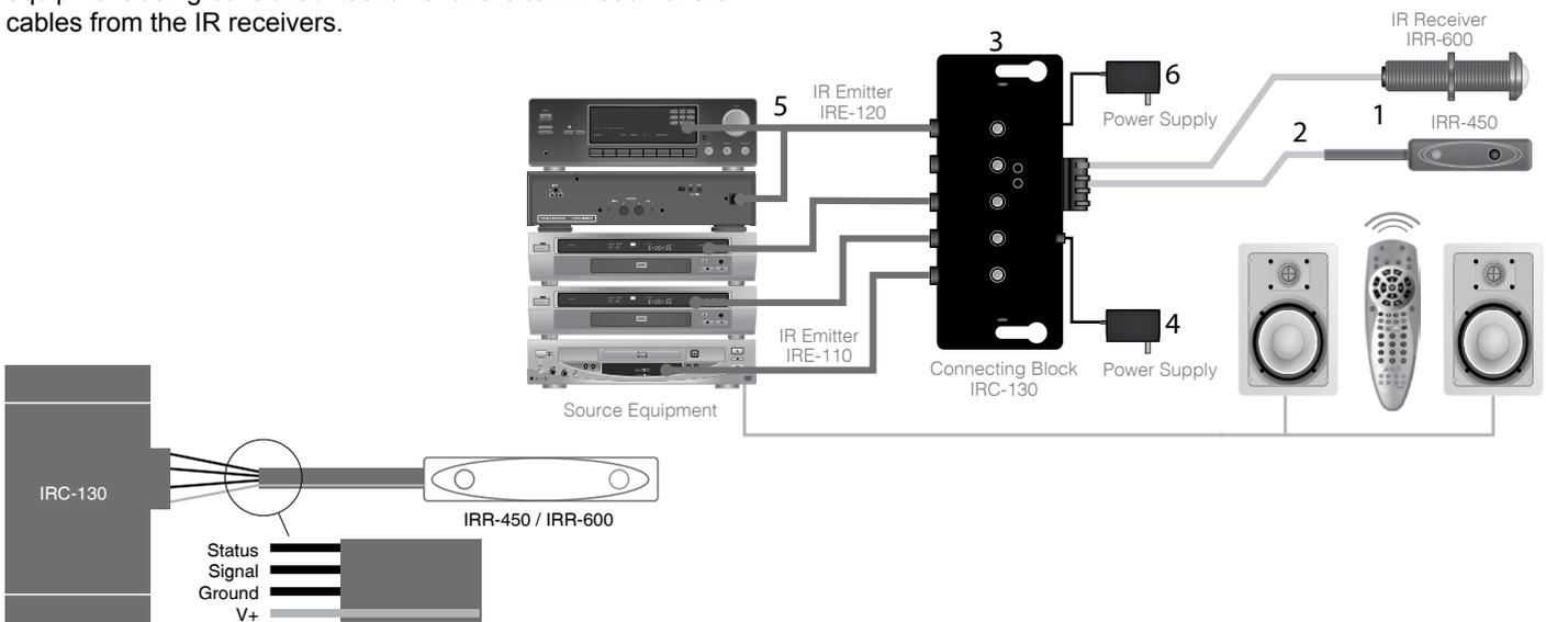
Wiring for connecting the IRR-450 & IRR-600 to the IRC-130
