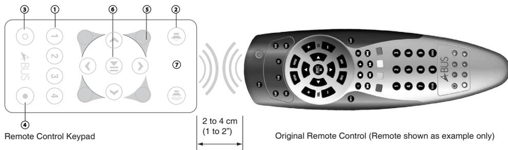
Note: This remote control keypad will learn most normal infrared commands using 38kHz and 56kHz carriers from typical remote control handsets. Some manufacturers codes do not comply with common infrared standards and may be difficult or impossible to learn and repeat.
