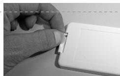
2. Pinch sliding tab and pull battery cage out simultaneously
